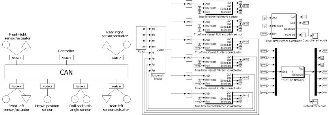
Figure 2. Simulated architecture. Left : schematic view - Right : implementation in TRUETIME
