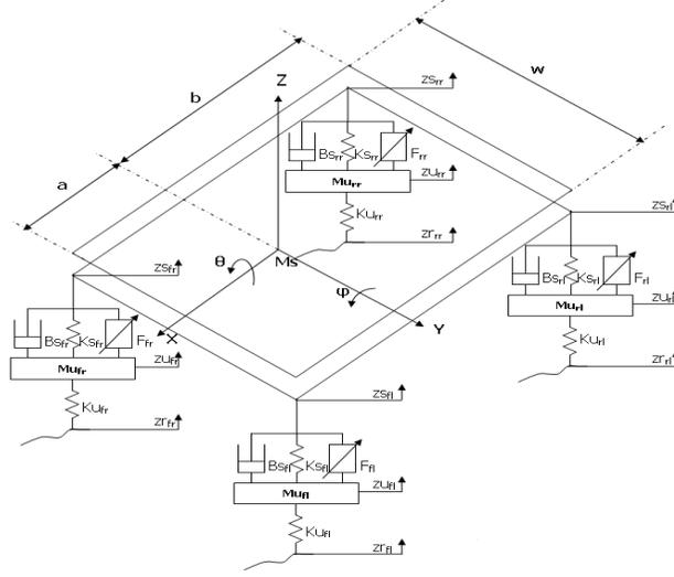
Figure 1. Model of the full vehicle
