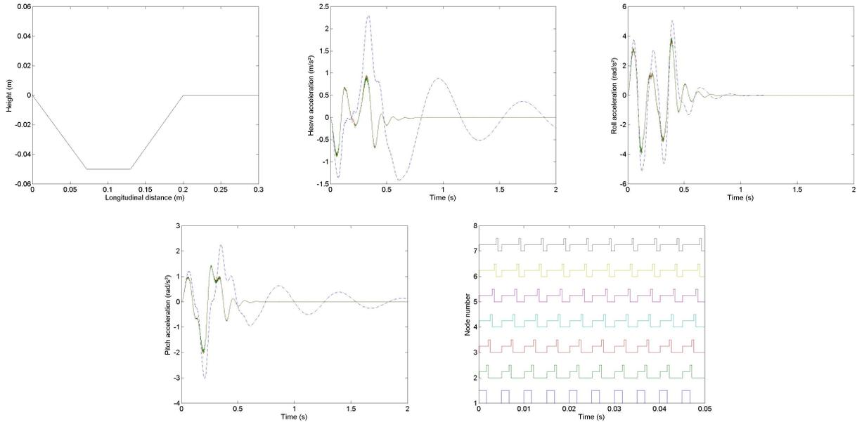
Figure 3. “Chunk hole” road disturbance, heave, roll and pitch accelerations of the sprung mass and network schedule. In the network schedule plot, a low signal means idle, a medium signal means waiting and a high signal means sending
