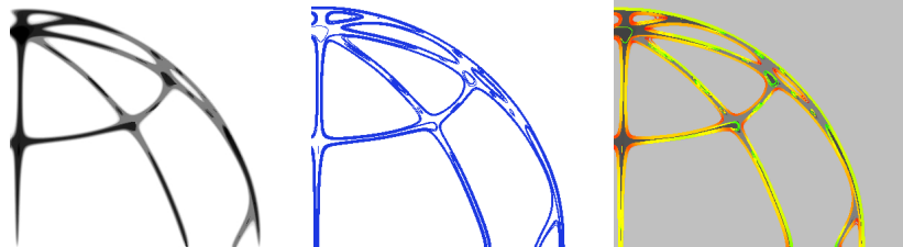
Figure: LLAS evolution, affine smoothed level lines and curvature map after filtering.
