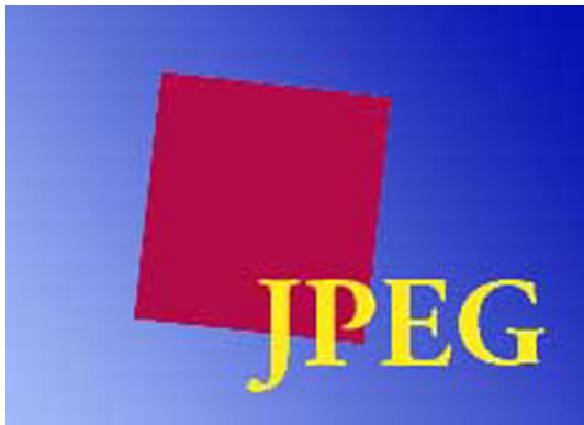
Figure: Original image, suffering of JPEG artifacts such as Gibbs oscillations, staircase noise along curving edges and checkerboarding.
