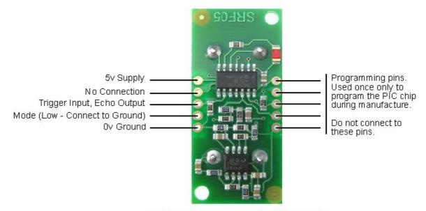
Connections for single pin Trigger/Echo Mode
