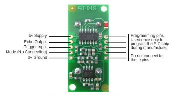
Connections for 2-pin Trigger/Echo Mode (SRF04 compatible)
