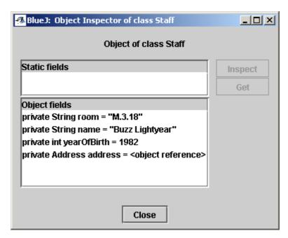
Figure 11: Inspection with object reference
